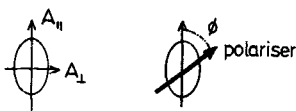
Figure 1. The definition of the polarizer angle, \phi , with respect to the parallel and perpendicular absorbances of the dye molecule.
